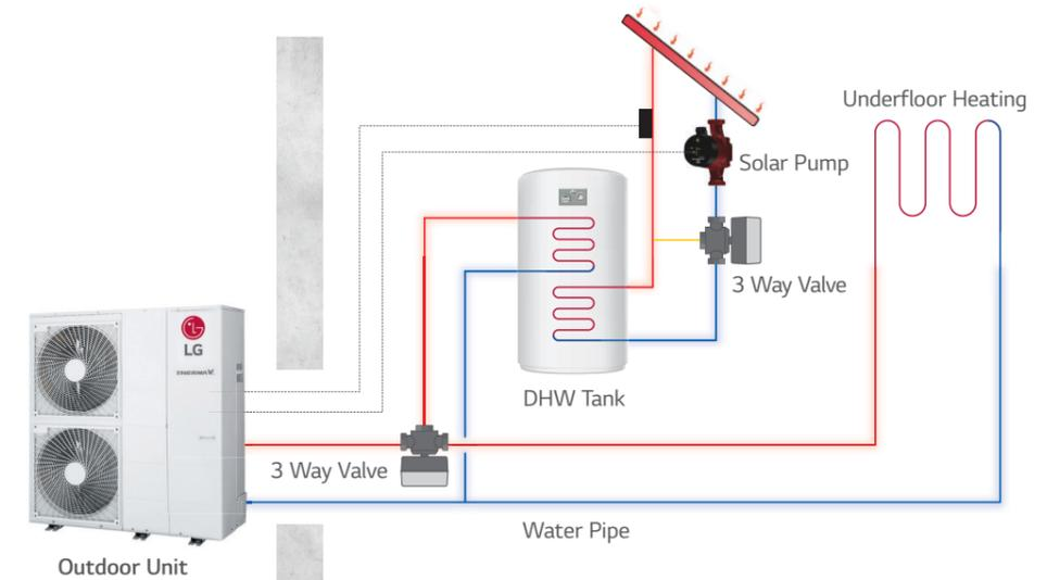
\* Mandatory accessory : Solar Thermal Kit (PHLLA) is required except for R32 Hydrosplit which needs PT-1000 type sensor (field supply).
