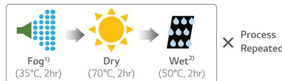
Test process is conducted according to ISO 14933.
