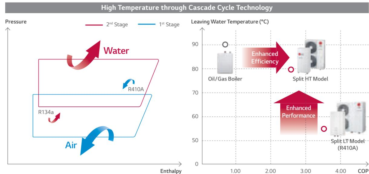
\* Condition for HT model : Outdoor air temp. 18°C, Entering water temp. 70°C
