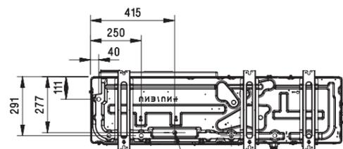
3-ID Ø 20 holes for drain connection
