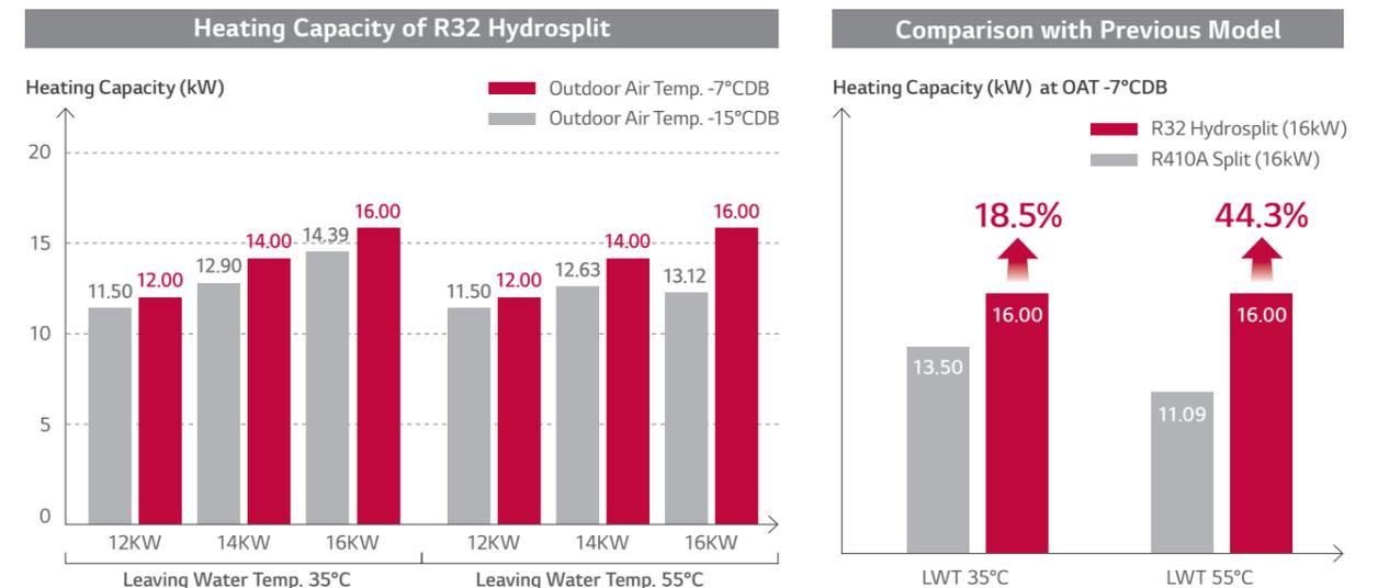
1) Normal : Outdoor air temperature 7°CDB / 6°CWB, Water outlet temperature 35°C
