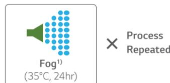
Test process is conducted according to ISO 9227.
