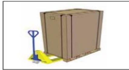
For the transportation, the heat pump is fix on the pallet and cover with a carton box.
