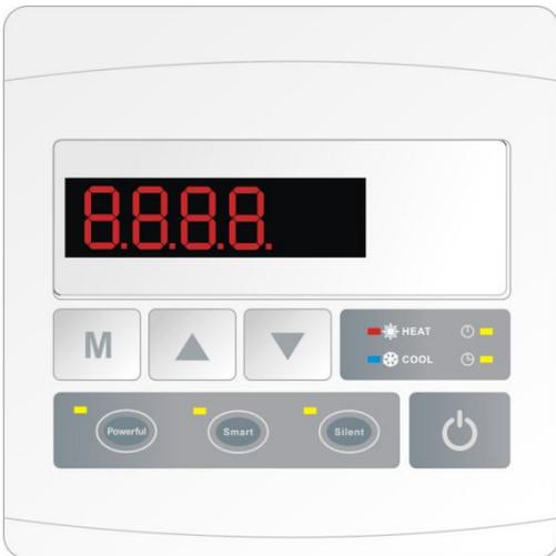
**NOTE:** Every time, when the heat pump connects to the power, the LED display shows a code for 3 seconds which indicates the heat pump model.
